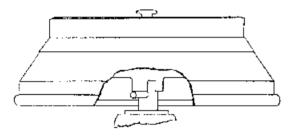
Figure 2: Motor shaft and rotor mounting hole – wrong!
